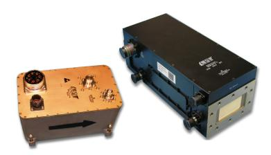
CPI Electron Device Business provides the capability to combine the LNA into a single package with the receiver protectors.
